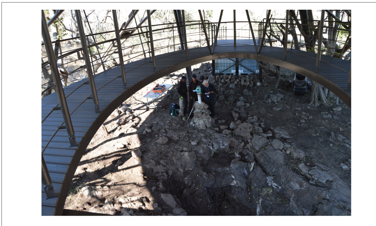
Figure 1: The use of conventional coordinate capture methods during excavations at Malapa Cave, Cradle of Humankind. The excavators are using a Nikon NPR-352 total station mounted on a known-position survey point to record the position of fossil material recovered during the excavation process. Site coordinates ( x , y and z ) are converted to geo-reference coordinates (easting, northing and height above sea level in the WGS 84 map reference system) by the total station.
