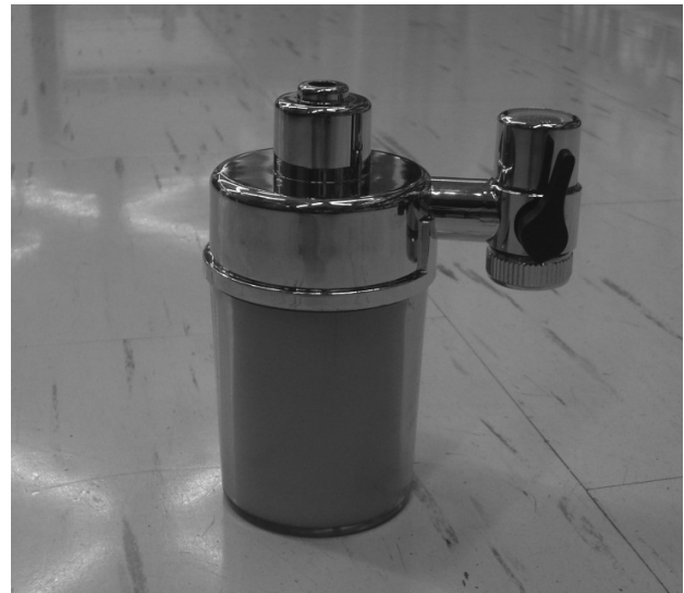
Figure 2: Mini tap filter – a point-of-use water-treatment device – which was used to collect biofilms.
