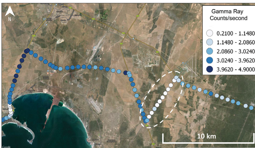
Figure 7: A Google Earth image indicating the relative uranium concentrations on tared roads of the West Coast of South Africa. The colour graded overlay displays the gamma ray counts in the region of interest around the 1764.5 keV gamma ray emission.
