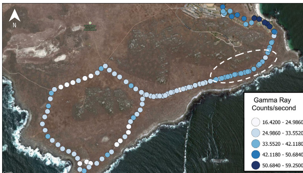
Figure 4: A Google Earth image indicating the relative uranium concentrations in the Saldanha Bay nature reserve, South Africa. The colour graded overlay displays the gamma ray counts in the region of interest around the 351.9 keV gamma ray emission.
