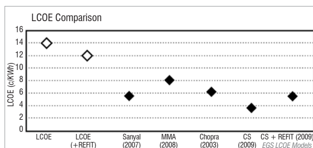
Figure 5: Graph comparing the calculated levelised cost of electricity (LCOE) of this study (white points) with the LCOE of other enhanced geothermal systems (black points).
