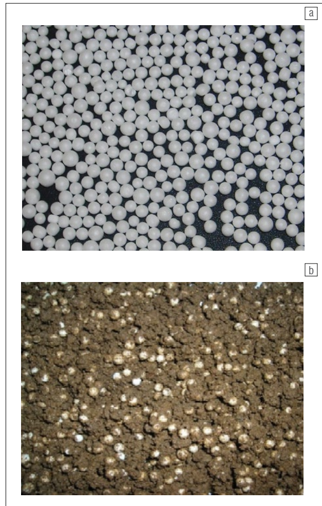
Figure 1: (a) Expanded polystyrene beads and (b) a mixture of expanded polystyrene beads and silty sand.
