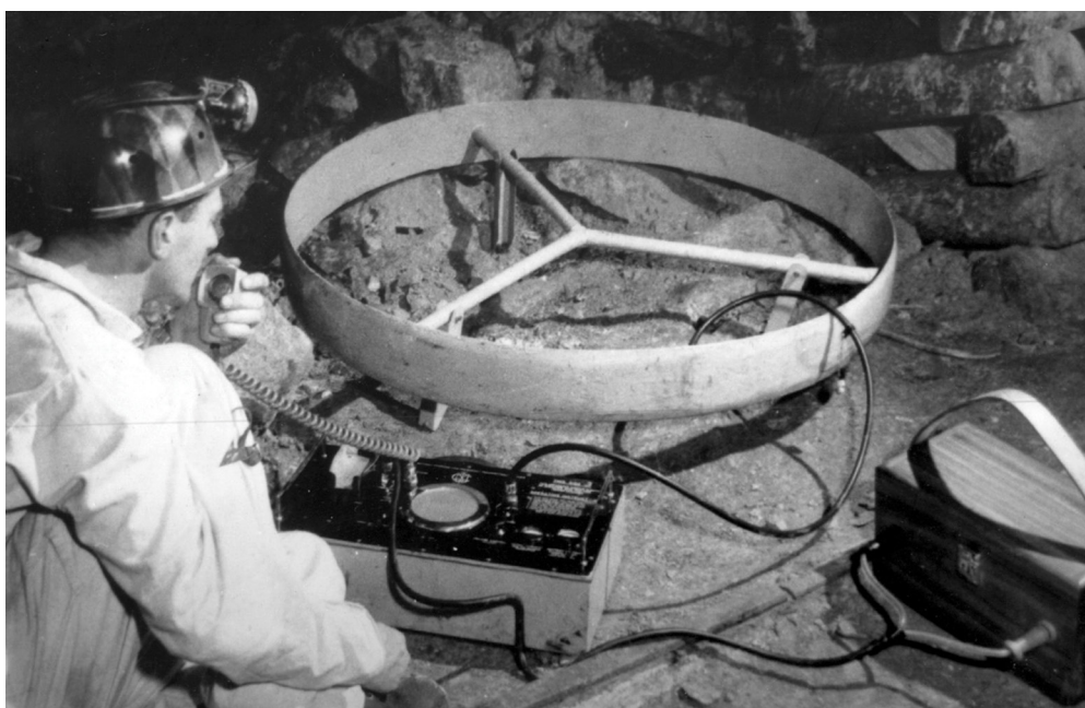
Figure 3: The fresh-air base radio equipment, its battery and multi-turn loop antenna.
