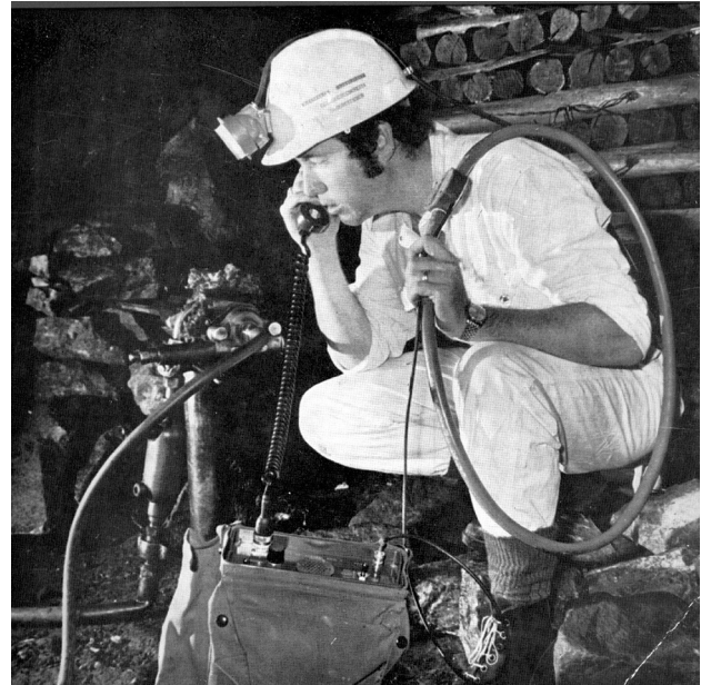
Figure 5: The single-sideband 335 kHz solid-state transceiver with its elliptical loop antenna.
