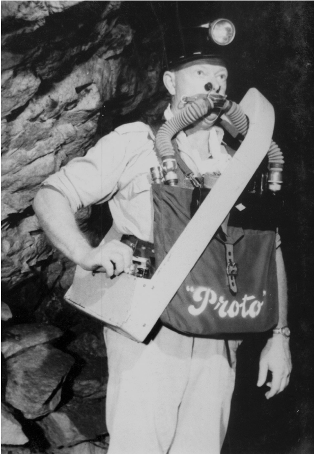
Figure 4: A brigadesman, using Proto breathing apparatus, with the portable radio equipment slung across his chest.
