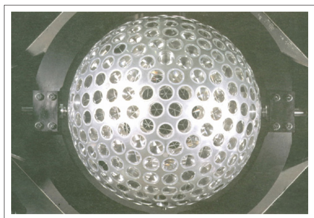
FIGURE 1: The satellite LAGEOS 1 contains an array of retroreflective mirrors covering its surface.
