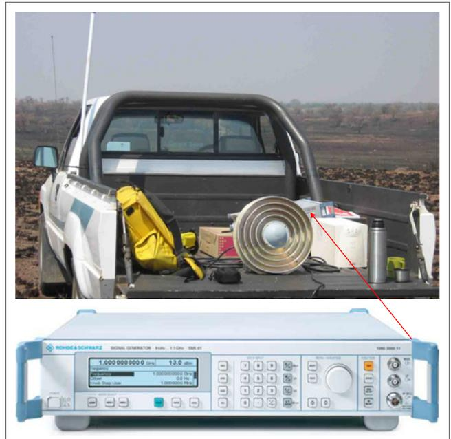
**FIGURE 1:** The jammer set-up used. A passive choke ring GPS receiver antenna was used as the transmitting antenna and matched the impedance of 50  $\Omega$  of the signal generator on both L1 and L2 frequencies.
