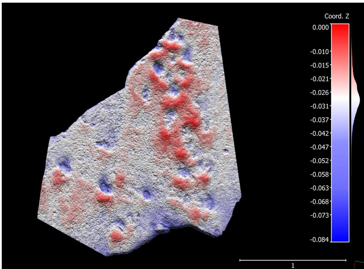
**Supplementary figure 1:** Photogrammetry colour mesh of the Site 2 epirelief surface, using 168 images. Photos were taken an average of 67.2 cm from the surface. The reprojection error is 0.372 pix. Vertical and horizontal scales are in metres.
