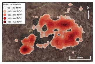
**Figure 6:** Heat map of the estimated radon potential overlaid on a Google Earth image of Baviaansberg.
