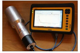
Figure 1: The Nal(TI) scintillation detector with a 7.62 x 7.62 cm crystal coupled to the scintiSPEC Multi-Channel Analyser and connected to the Trimble Yuma Rugged tablet computer via the USB connection.
