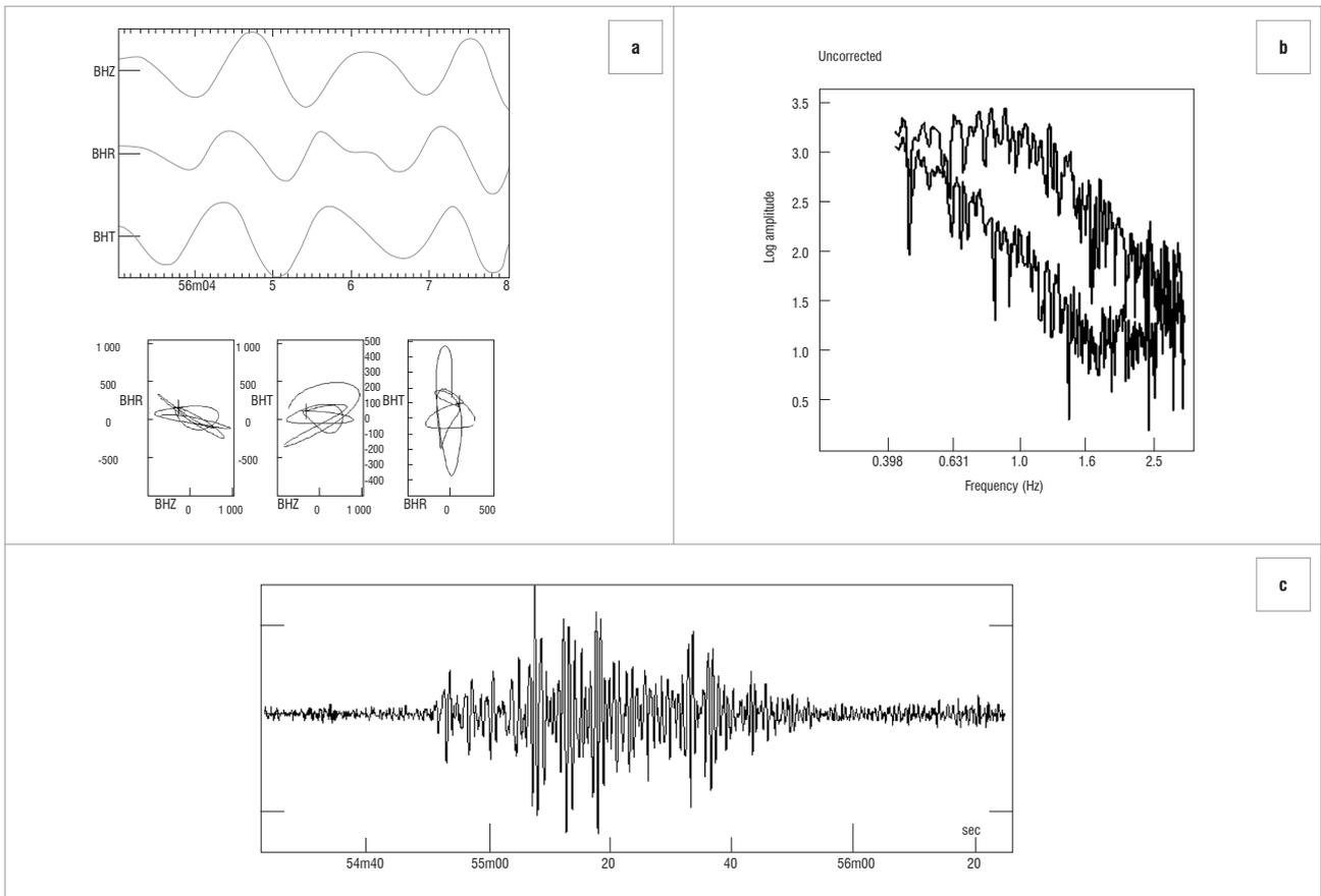
**Figure 4:** Detailed view of signal S1 showing (a) the particle motion, (b) the spectra of the signal and (c) the time series.
