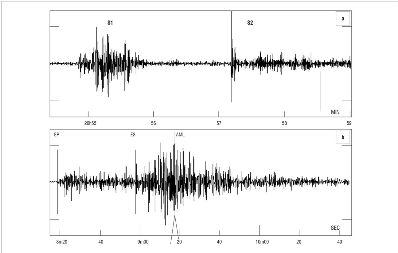
**Figure 3:** (a) Signal recorded at the Mussina station during the passage of a meteor on 21 November 2009. (b) Signal of a magnitude 3.2 earthquake originating in Mozambique recorded on 04 March 2009 at 17:08 (UT).
