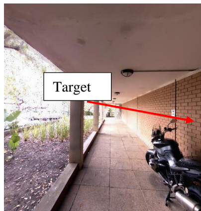
Figure 4: Sample of Terrestrial Laser Scanner Targets placed on North wall
