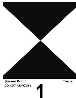
Figure 4: Sample of Terrestrial Laser Scanner Targets placed on North wall
