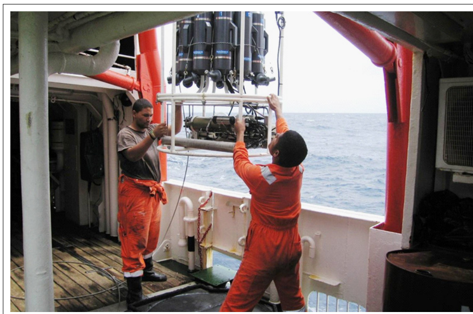
Figure 1: Crew members of the research vessel FRV Algoa preparing to launch a rosette sampler with conductivity-temperature-depth, oxygen sensors and fluorometer during the ACEP II cruise of October 2009
